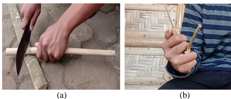
Fig. 3 (a) Seltok making process from a segment of bamboo; (b) Seltok Handle
