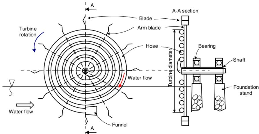
Figure 1. Spiral pumping wheel schematic
