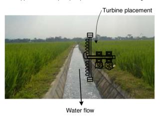
Figure 2. An example of a spiral pump mill application
