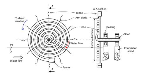
Figure 1. Spiral pumping wheel schematic
